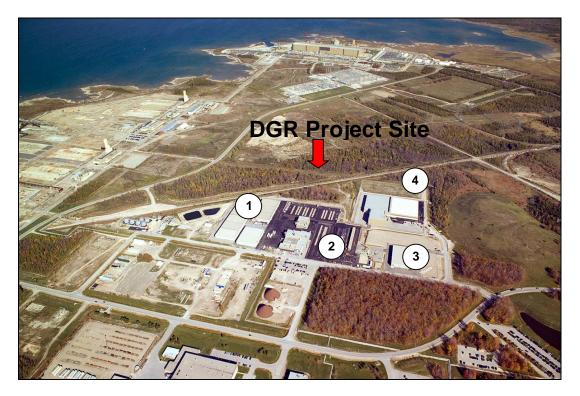
Figure 2-1. Aerial view of OPG's Western Waste Management Facility (October 2007); 1) Ten Low-Level Storage Buildings, 2) In-ground Containers for ILW, 3) Refurbishment Waste Storage Buildings, and 4) Western Used Fuel Dry Storage
