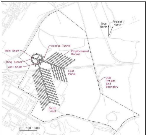
Figure 4-1. Conceptual layout of a repository to accommodate OPG's L&ILW
