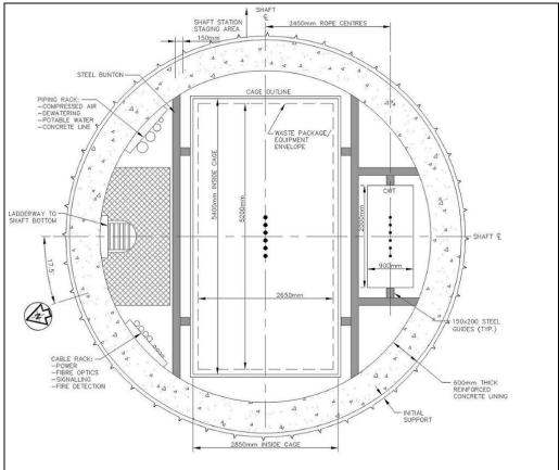
Figure 4.2. Conceptual layout of DGR Main Shaft
